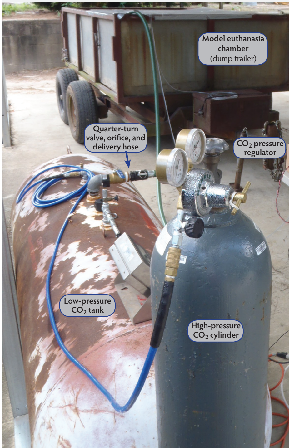
Figure 3: A prototype CO 2 application system assembled and used to verify the performance of the swine euthanasia system illustrated and described in figures 1 and 2. A pressure-relief valve has been added to a used propane tank to serve as the low-pressure CO 2 tank. An orifice plate (Figure 4) was included in the discharge hose to control the CO 2 gas flow into the dump trailer used as a model euthanasia chamber.
