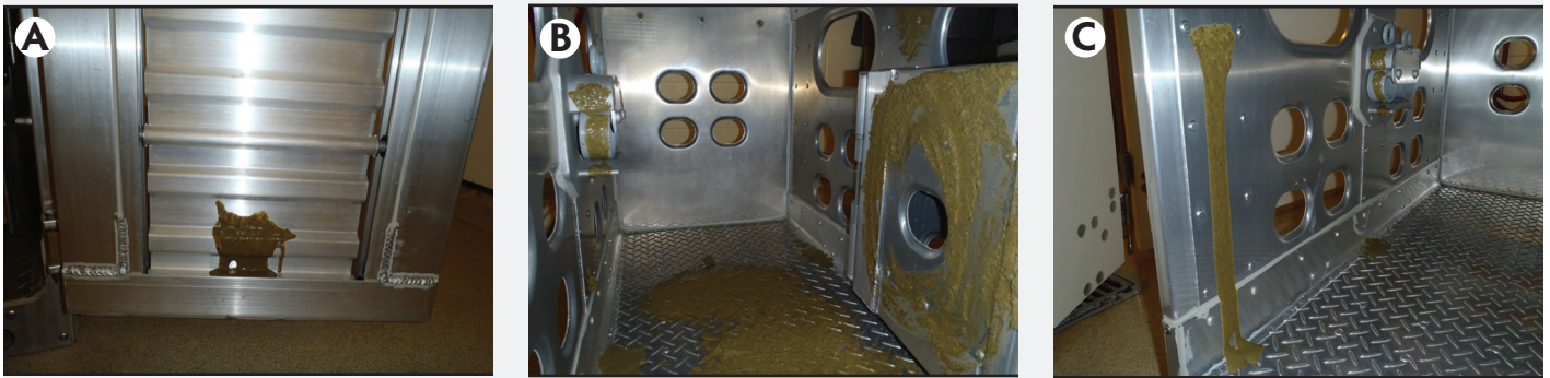
Figure 4: After contamination, model trailers in Objective 1 (study described in Table 1) were washed with a high-pressure washer (1500 pounds per square inch) using cold water. Shown are a contaminated model trailer prior to washing (Panel A) and model trailers after high-pressure washing (panels B and C).
