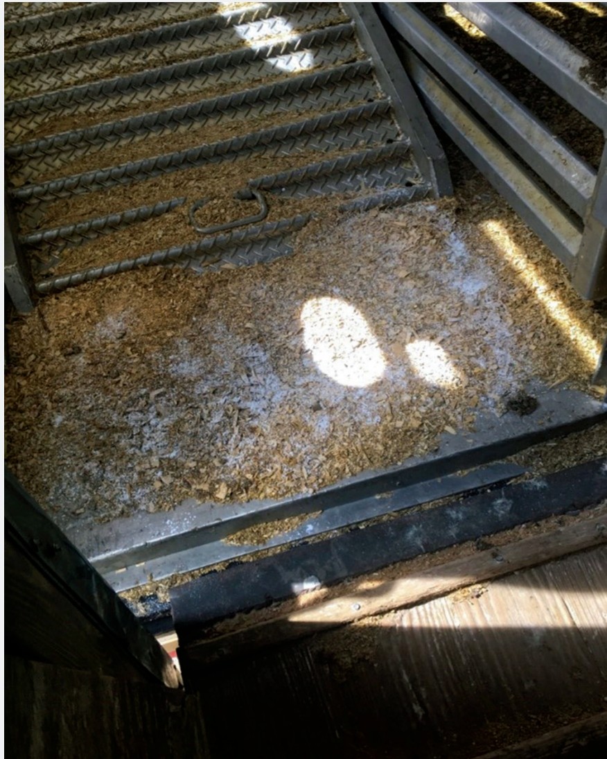
Figure 4: The mixture of fluorescent powder (Glo Germ), wood chips and obstetrics gel placed just inside the roll up door of the livestock trailer. The fluorescent powder appears white in sunlight and fluoresces when the primary light source is long-wave ultraviolet.
